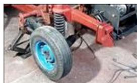
Fig. 11. Tire lifted to get the neutral condition.
