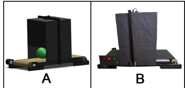
Fig. 4. (A) 3D Model of the conveyor belt system and (B) Conveyor belt system built for the project.
