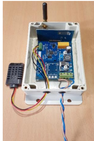
Fig.7. Sensor node inside the enclosed
