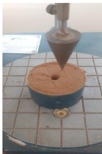
Fig. 2. Determination of liquid limit using cone penetrometer method
