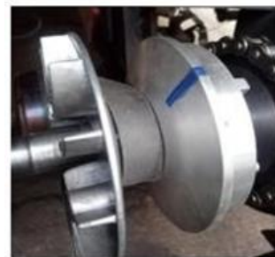
Fig. 12. Ink mark to determine the belt rising level
