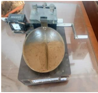
Fig. 1. Determination of liquid limit using Casagrande method
